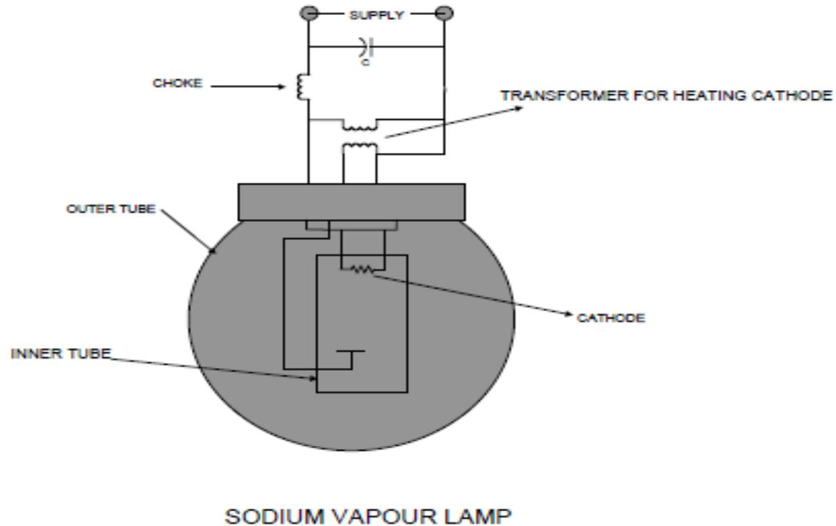
A choke is provided for stabilizing the electric discharge and a capacitor for power factor improvement.
