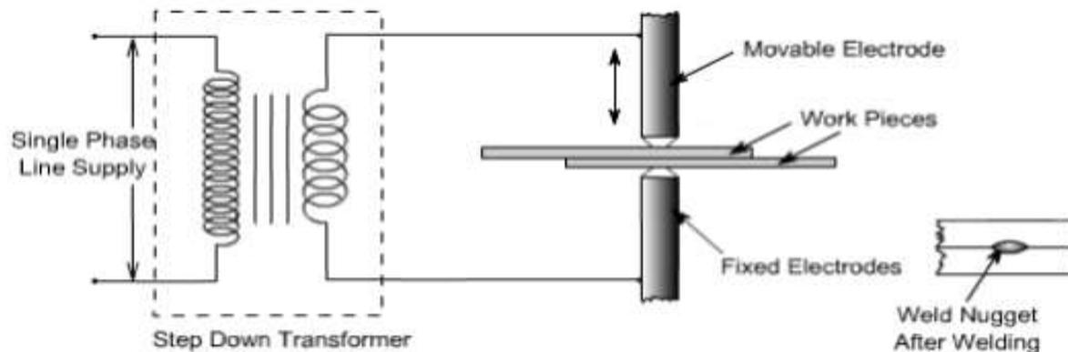
Principle of Resistance spot Welding
