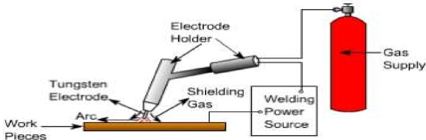
Schematic Diagram of TIG Welding System.
